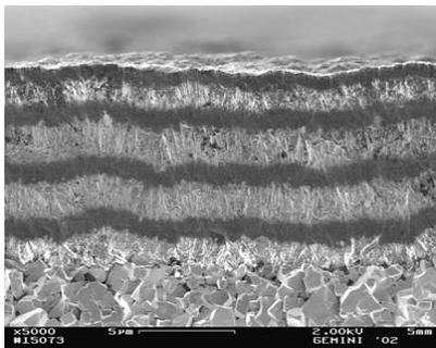
Picture 1: multilayer diamond coating (picture of CemeCon AG)
