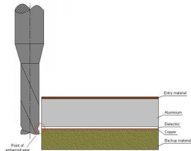
Picture 5: increased tool wear caused through the ceramic layer
