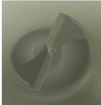
Picture 2: diamond coated drill after 7000 hits
